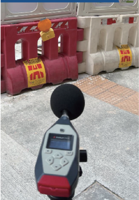
定期監測工程發出的噪音 Monitored Noise Level of Foundation Works Regularly
